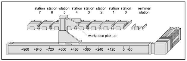
The horizontal movement is implemented using an NC axis controlled by COMPAX. A pneumatic cylinder, which is controlled by COMPAX using a double solenoid valve, raises and lowers the workpiece pick-up. COMPAX performs all the functions required without superordinate control.
